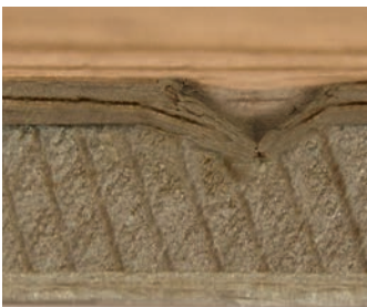
Standard, ready-made parquet with traditional spruce | fir middle layer made of grown wood
