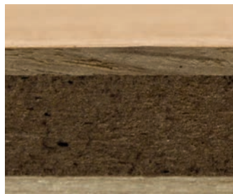
Modern ready-made parquet with dimensionally stable middle layer made of special HDF
